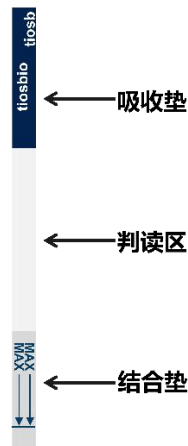
Figure 1. Schematic Diagram of Disposable Nucleic Acid Detection Test Strip Structure
